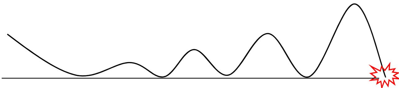
In an aircraft like the jeans, a PIO can occur when the glider touches down on the main-wheel and bounces back into the air. The pilot pitches the nose down and the glider strikes the ground, resulting in the nose pitching up rapidly.
